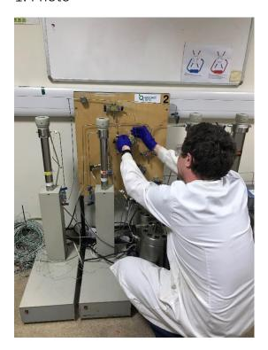
Operation of the biological flow apparatus designed to monitor the interactions of microorganisms, geological/engineered materials, fluids and gases
