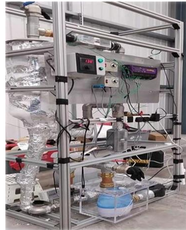
Figure 2 BEIC hanger Thermochemical energy storage demonstrator (5kW/50kWh)
