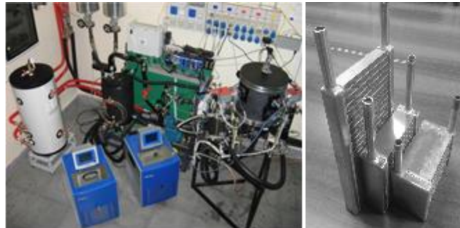
Reactor/adsorber testing bench.
