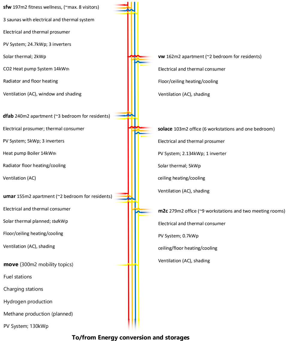
Figure 2: Overview of energy-related systems and components in each of the NEST modules and at the Empa mobility demonstrator move, all interconnected via several networks (3 electrical, 3 thermal, 2 gas [not shown]). The NEST module names are abbreviated in bold letters.
