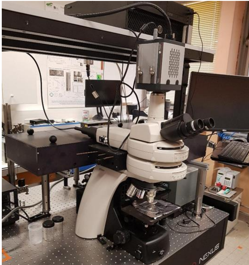
Figure 1: the upright microscope coupled with Raman spectrometer.
