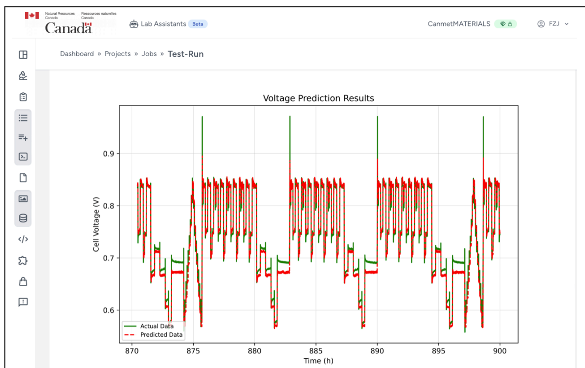
Figure 5. Illustration of predictive power of the CNN-LSTM model for PEMWE, deployed in ViMi platform.
