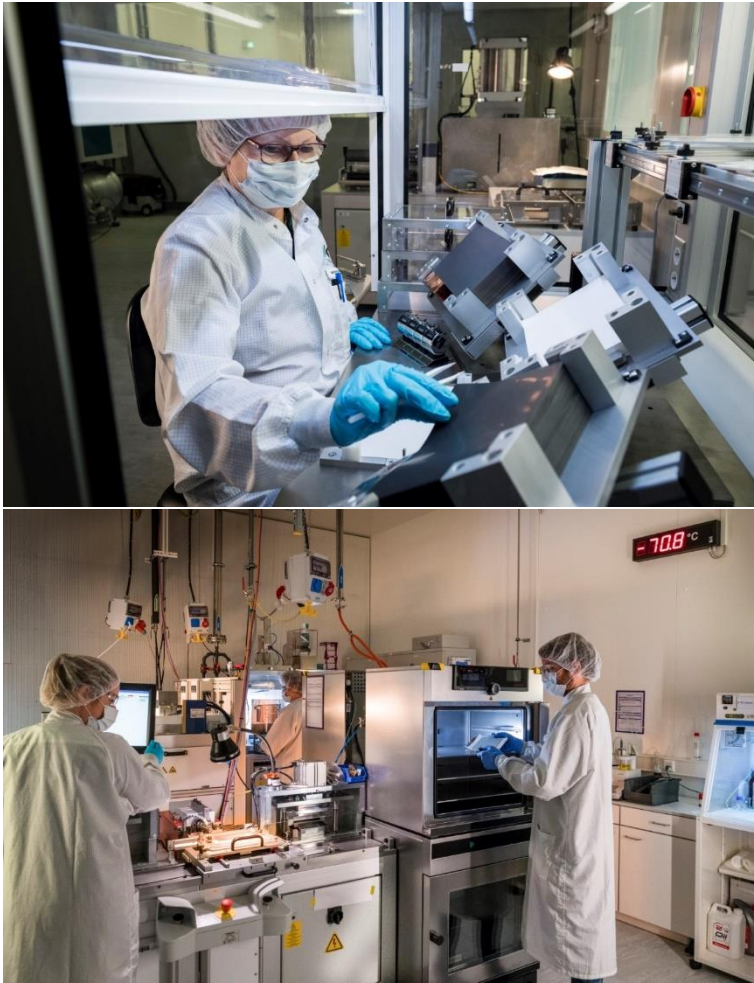
Figure 2 Assembling of large-format pouch cells in the dry-room at the Battery Technology Center at KIT.
