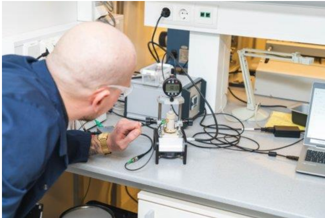
Figure 2. Ophelia cell with gauge meter for thickness variation measurements
